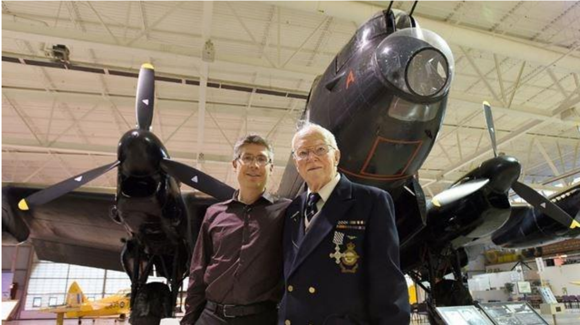
Figure 19: Alex Campbell and Lancaster bomber showing the forward turret and the bomb aimer's position in the Perspex cupola.
